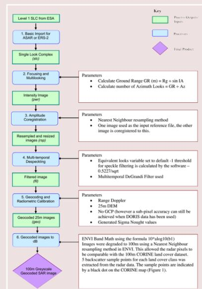
Figure 3 - SAR preprocessing steps in SARscape 4.2 to produce the intensity images adapted from (Kitmitto et al., 2007).
